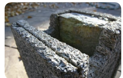
Concrete insulated with wood waste
